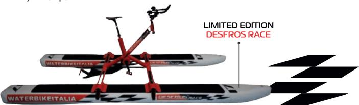
Dimensions: 400 cm x 140 cm. Weight: 36 kg. Maximum recorded speed: 17 km/h. Average speed at 80 pedal strokes per minute: 8 km/h. Maximum weight capacity: 140 kg on the saddle and 200 kg overall with the sun lounger mattress.
