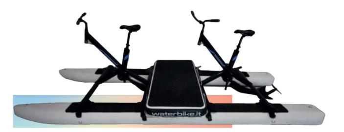
Dimensions: 400 cm x 140 cm Weight: 48 kg Maximum recorded speed: 12 km/h. Average speed at 80 pedal strokes per minute: 7.5 km/h.
