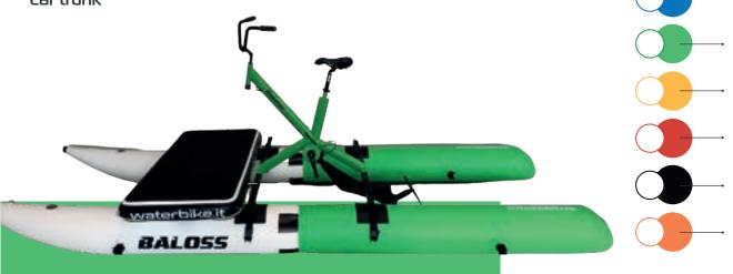
Dimensions: 420 cm x 140 cm. Weight: 27 kg. Maximum recorded speed: 16 km/h. Average speed at 80 pedal strokes per minute: 8 km/h. Maximum weight capacity: 140 kg on the saddle and 200 kg overall with the sun lounger mattress.
